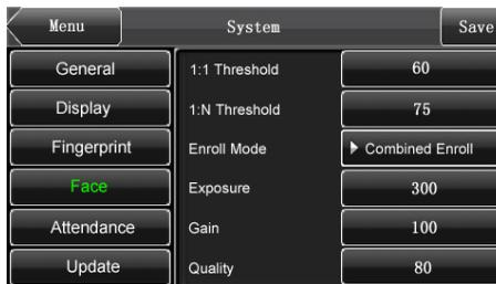
**1: 1 Threshold:** This parameter is used to set the threshold of matching between current face and the facial template enrolled in the IFACE terminal in the 1:1
