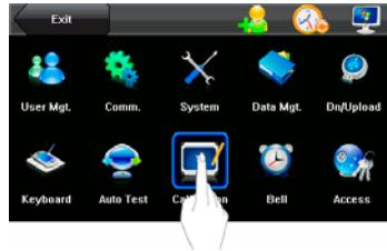
2. Press [Calibration] on the main menu interface to display the screen calibration interface.
