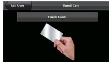
3. If the card passes the verification, the IFACE terminal displays a prompt message “Read Successfully! Card No.: \*\*\*\*\*”, as shown in Figure 3 on the right, and returns to the [Add User] interface. Press [Card] to display the enrolled card number as shown in Figure 4 on the right.
