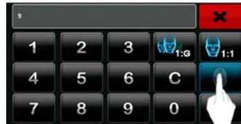
3. Press your finger on the fingerprint collector by adopting the proper finger placement. For details, see *1.1 Finger Placement*.
