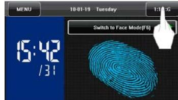
2. Enter user ID and then press the "Fingerprint" icon (Figure 2 on the right) to enter 1:1 fingerprint recognition mode. If the prompt "Unregistered user!" is displayed, the user ID is nonexistent or the user ID bearer has not enrolled his/her fingerprint.
