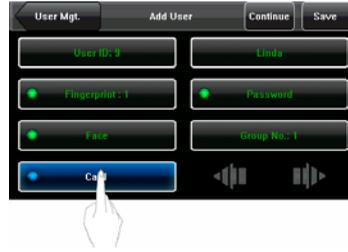
2. The [Punch Card!] interface pops out as shown in Figure 2 on the right. Swipe your ID card properly in the swiping area. For details, see “1.6 Appearance of the IFACE Terminal”.
