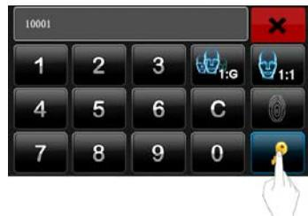
3. Enter the password and press the “OK” icon to start the password comparison, as shown in Figure 3 on the right.
