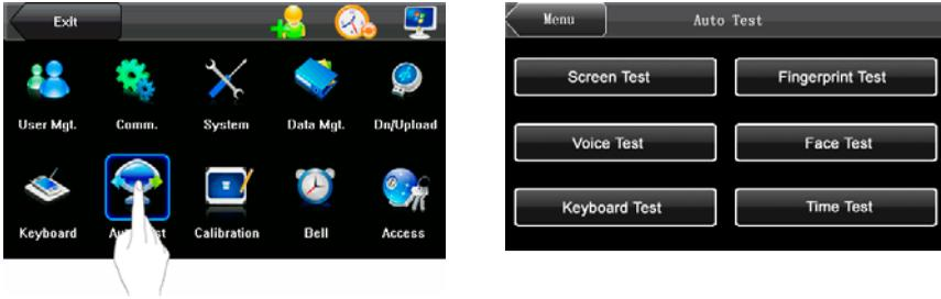
**Screen Test:** The IFACE terminal automatically tests the display effect of the color TFT display by displaying full color, pure white and pure black and checks whether the screen displays properly. You can continue the test by touching the screen or exit it by pressing [Auto Test].
