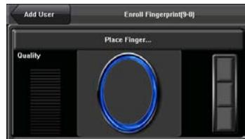
3. Place the same finger on the fingerprint collector for three consecutive times correctly. If the enrollment succeeds, the system will display a prompt message “Enrolled Successfully” and automatically return to the [Add User] interface (as shown in Figure 4 on the right). If the enrollment fails, the system will display a prompt message and return to the [Enroll Fingerprint] interface. In this case, you need to repeat the operations of step 2.
