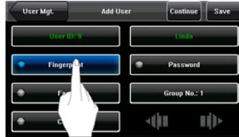
2. On the displayed [Enroll Fingerprint] interface (as shown in the Figure 2 on the right), place your finger on the fingerprint collector properly according to the system prompt. For details, see “Finger Placement”.
