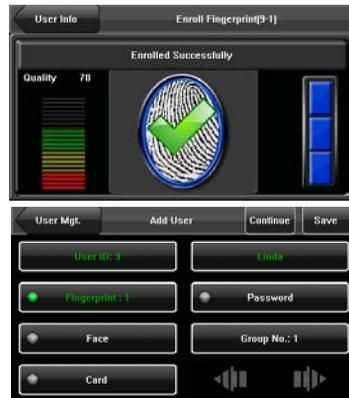
4. You can back up the enrolled fingerprint of a user by pressing [Fingerprint]. A user can enroll 10 fingerprints at maximum.
