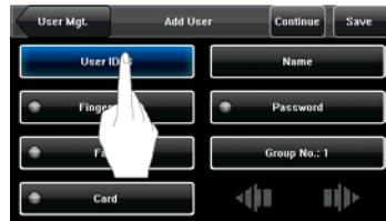
2. On the displayed keyboard interface, enter a user ID and press <OK> as shown in Figure 2 on the right. If a prompt message "The user ID already exists!" is displayed, enter another ID.
