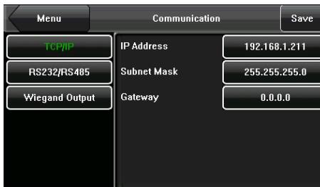
**IP Address:** The IP address is 192.168.1.201 by default and can be changed as required; the IP address of the IFACE terminal and that of the PC cannot be duplicated.
