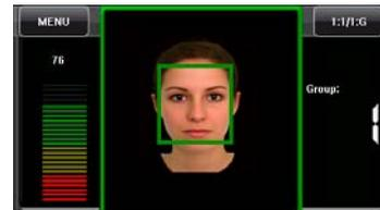
4. If the verification is successful, an interface as shown in Figure 4 on the right will be displayed. The system will return to the main interface if the verification is not passed within 20 seconds.
