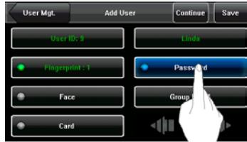
2. On the displayed keyboard interface, enter a password and press <OK> as shown in Figure 2 on the right. Re-enter the password according to the system prompt and then press <OK>.
