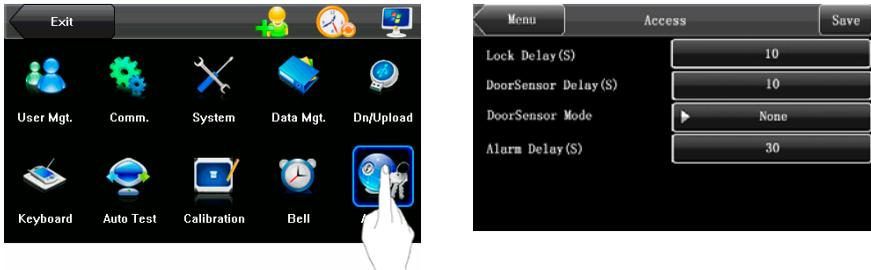
**Lock Delay:** indicates the duration for the IFACE terminal to place the electric lock in open state. (Value scope: 1–10 seconds)
