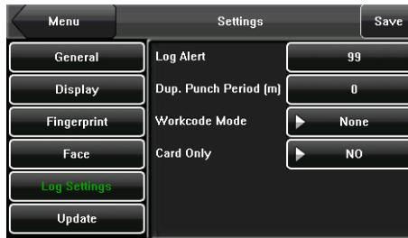
**Log Alert:** When the available space is insufficient to store the specified number of attendance records, the IFACE terminal will automatically generate an alarm. (Value scope: 1–99)
