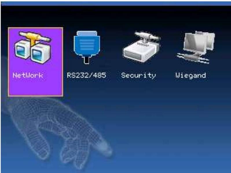
From within the Comm Menu, scroll with the ◀/▶ keys until **Network** is highlighted. Press the **OK** key to accept.
