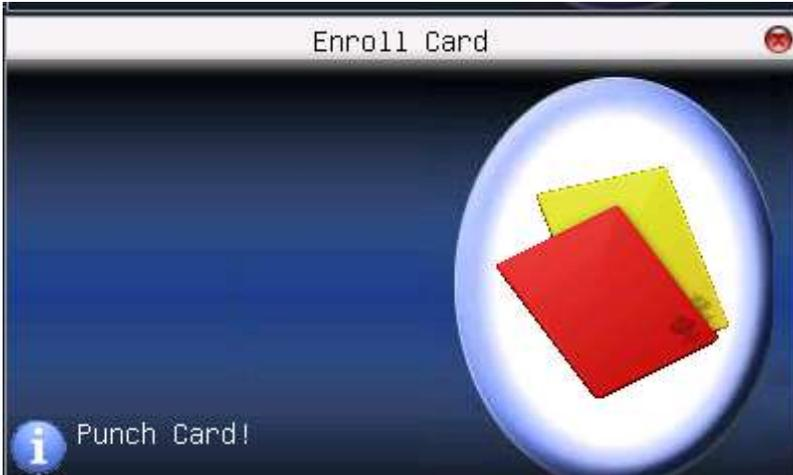
Flash the card near the keypad of F18 reader, press OK key to save after the device reads and displays the card number.
