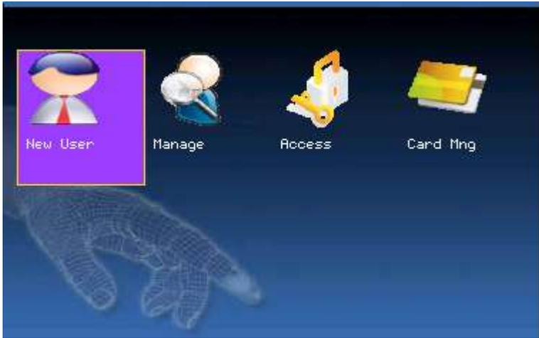
Scroll with the ▲/▼ keys and highlight **Manage**. Then press the **OK** key to open the User Manage screen:
