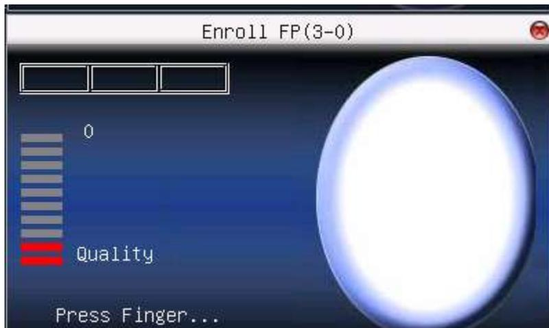
Place the finger you wish to enroll on the sensor, ensuring the finger is placed flat and centered. Hold the finger still for at least two full seconds until the F18 prompts with a beep to remove it. You will then be prompted to repeat the process 2 more times, **each time using the very SAME finger.**
